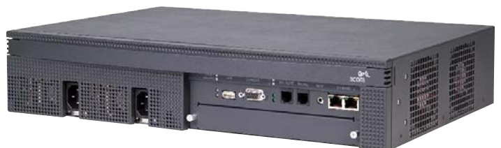
Standards-based 3Com V3001R platforms offer dual redundant power supplies (standard) and hard drives (optional) to maximize operational uptime.
